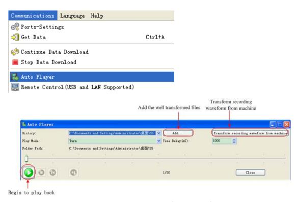
Figure 4-12: Play back waveform by software
