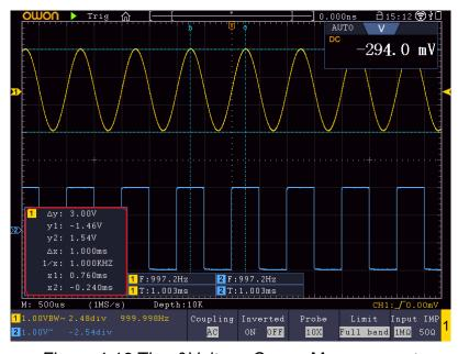
Figure 4-16 Time&Voltage Cursor Measurement
