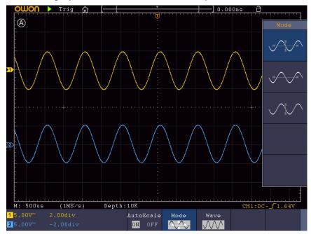
Figure 4-17 Autoscale Horizontal-Vertical multi-period waveforms
