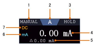
Figure 6-3 Multimeter Information Window
