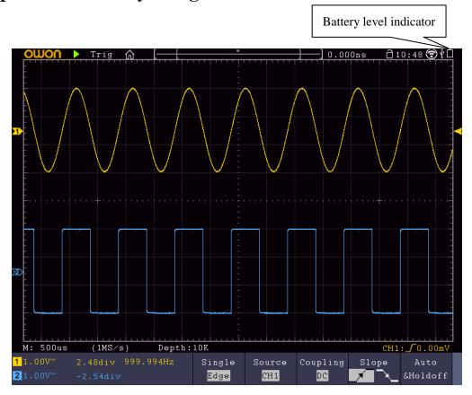
Figure 12-1 Battery level indicator
