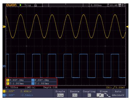
Figure 4-13 Automatic measurement
